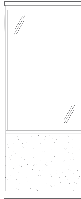
CS1G1: HALF Half glass panel Available in: Single 6 mm Single 10 mm
